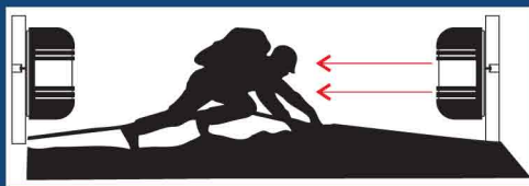
When the signal is blocked, the detector sends alarm information to the control panel
